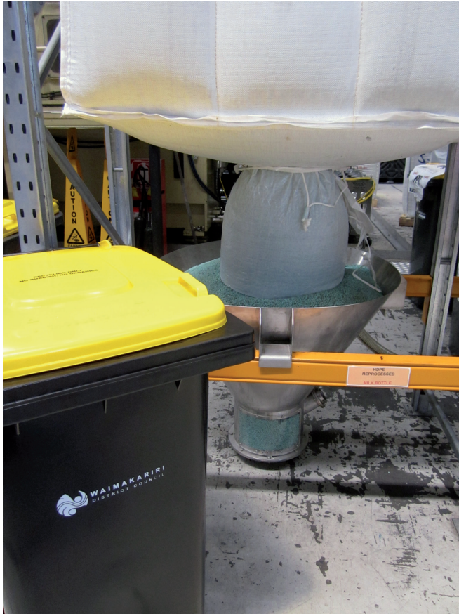
A Waimakariri recycling bin alongside a hopper of the milk bottle material used in its manufacture. Comspec supplied the milk bottle material.
